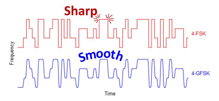
By smoothing the frequency transitions ▲, GFSK significantly reduces the skirts (sidebands) on the two simulated signals shown on the right of this spectrum plot ▼ narrowing the FT8 bandwidth by a remarkable ~80% at the -80 dB level. Even unsmoothed, FT4 and FT8 sigs are *much* narrower than RTTY.
